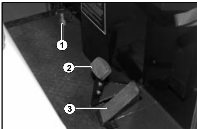
Foot Controls 1. Dimmer Switch 2. Brake Pedal 3. Foot Throttle Pedal
