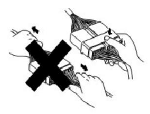
2.Connectors can be removed by pressing or pulling lock lever.
