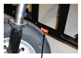
Place Jack In The Center Of Front Cross Tube Or On Either Side Of The Rear Subframe
